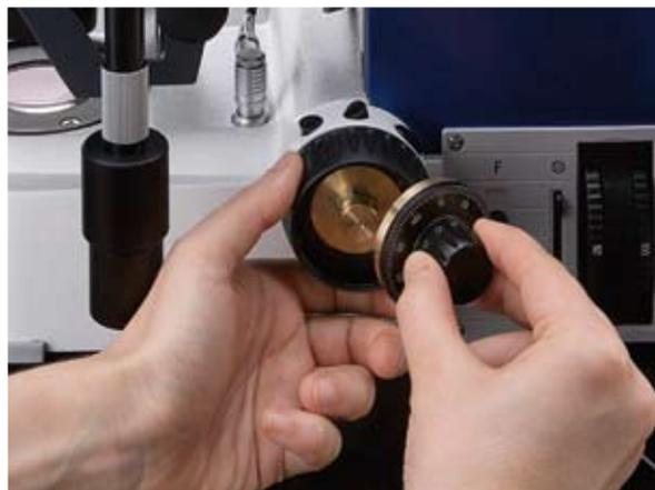
*Two different kinds of fine focus controls are available for the focusing drive in Axio Imager: They are interchangeable and can be used either on the left or the right hand side.*
