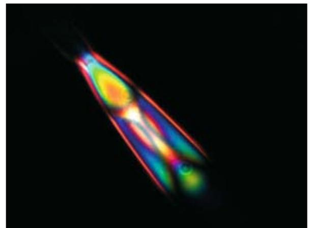
*Glass fiber filled with liquid crystal, linearly polarized transmitted-light
