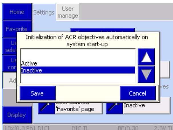
Fig. 4-109 Initialization of ACR objectives after switch-on
